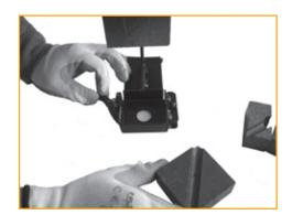
MM-PTX for cable or tape to earth rod (usually T shape) The piece has the diameter of the earth rod according to the requirement (MM-PT14, MM-PT16....), working only for this specific rod diameter (see mechanized earth rod diameters on section C.1 in this manual)
