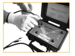
The electric contact between the clamp and the spike is essential. The clamp must not touch any other part of the cover. If the clamp becomes worn, just replace it (AT-100N kit Apliweld-E includes 5 of these clamps)
