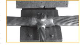
Take the welded conductors out of the mould
