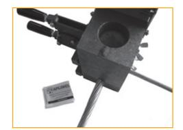
DO NOT pour the whole contents of the package on the tablet. It would make the ignition more dangerous and will damage the spark lighter (**AT-060N**). The powder path is aimed to provide an easy and safe ignition.
