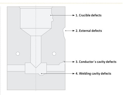
Remember that the sections of the conductors are the marked on the mould. Consider also the right diameter for the section. Otherwise use **AT-072N** Adapter Sleeves in case of cables. Conductors must keep a convenient shape with no deformation, allowing the correct closure of the mould/clamp system.
